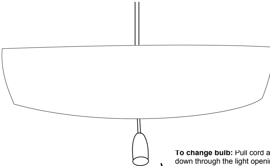
**To change bulb:** Pull cord and light socket down through the light opening. Socket locks into edge of opening so the bulb can be changed.
